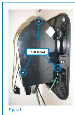
3. Remove the three (3) screws attaching the air inlet cover and remove it from the dryer. Save all three of these screws for later use in Step 10. (Figure 3)  ${\bf 4.}$  Remove the two (2) screws and one plastic housing retainer holding down the foot of the dryer. (Figure 4)
