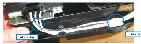
9. Attach Control Harness Connector to Control and route wires as shown in Figure 9. Make sure wires are installed under white clip on adapter. Connect green wire back on quick connect tab on bracket. Reconnect sensor to Control. (Figure 9)
